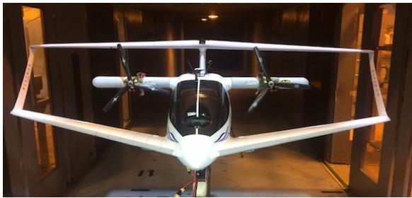
Figure 4: Elytron 4S UAV in the US Army 7x10 subsonic wind tunnel at NASA Ames Research Center.
