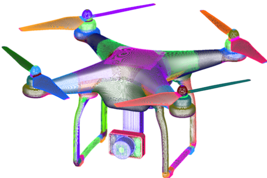
Figure 9: Overset surface grids for the complete DJI Phantom 3.
