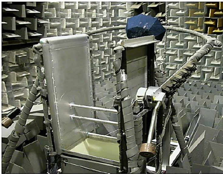
Figure 18: Tandem cylinder arrangement in Quiet Flow Facility (QFF) [1]
