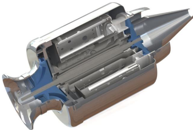
Figure 2. The model of KJ 66 engine in FloEFD.
